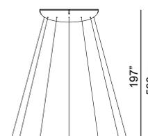
NOTE: The final shape of the luminaire may vary according to the length of the suspension cables.
